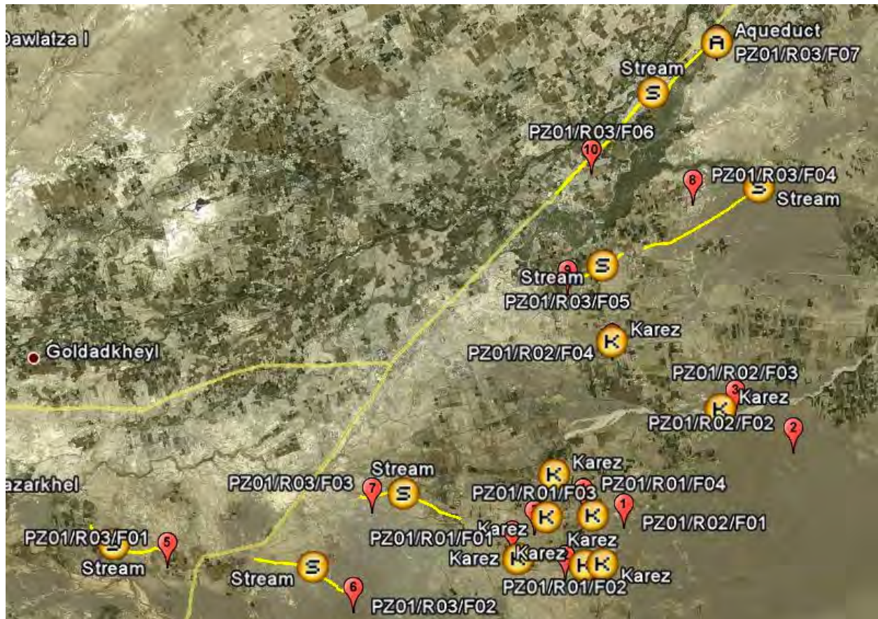
Figure 15 The location of karezes, streams/canals and aqueducts in Zurmat and the landforms where they can be found
