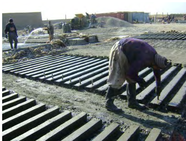
Inserting holes in trellis posts
